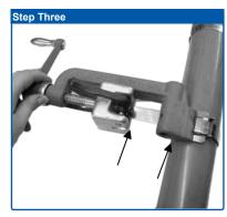
Place band in opening of tool nose and gripper block. Move into slot as far as possible, to avoid buckle sliding into tool nose. Tighten band clamp by turning the tension handle clockwise while holding band gripper tight against band. NOTE: The spring load of the band gripper is not intended to secure and prevent band from slipping during tension process.
