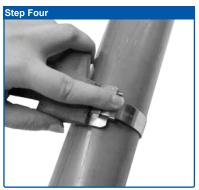
Place finger on BAND-IT Band at buckle bridge while tensioning with tool handle. When you feel BAND-IT Band stop moving through buckle as you are turning handle, maximum pressure is being exerted by the BAND-IT Band around object being clamped. Stop turning handle.
