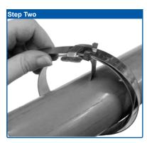
Continue band around object once more and again through buckle. Double banding develops a great deal more radial compression than single banding. Bend end of band under buckle.
