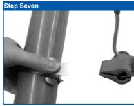
Remove tool, holding stub of band down with thumb.
