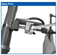
Roll tool over buckle, backing off with tension handle throughout entire rolling operation. Failure to back off with tension handle through-out entire course of rollover may result in breaking of band. There is no loss of tension as band released is used up in the bend.
