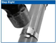
Hammer down buckle ears to hold band stub in place to complete BANDIT clamp
